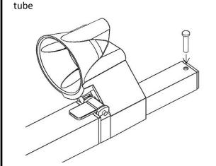
**4** Insert the lock with the head of the pin orientated with the cavity on the muzzle holder
