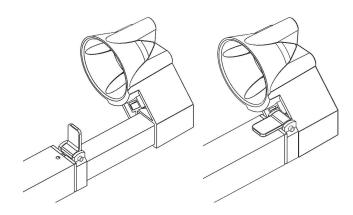
**Do Not** lift the stroke limiter lever unless both tubes are being held or the tubes will retract quickly
