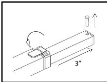
2 Carefully extend/pull the silver extension tube out about 3 inches, push the lever on the stroke limiter down to lock the tube from retracting and remove the lock pin
