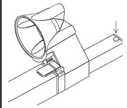
**5** Slide the muzzle cup out and over the lock pin head and tighten screw firmly
