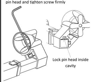
**6** While holding the muzzle cup and black extension tube, raise the lever on the stroke limiter and slowly let the tube contract
