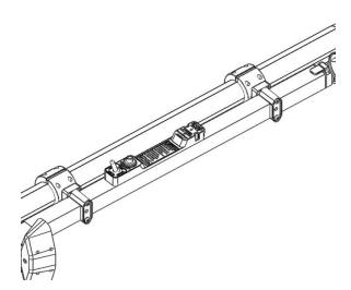
Slide and rotate the LS&B into its desired location and tighten the eight back clamp screws and the four upper clamp screws.
