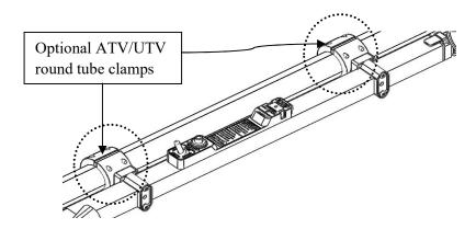
Measure the dia. of the tube and use the proper optional round tube clamps.
