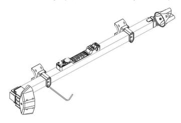
Place the U shaped upper clamp over the Locked Stock & Barrel and loosely attach to the lower clamp using the four longer screws. Do Not firmly tighten until installation is complete.
