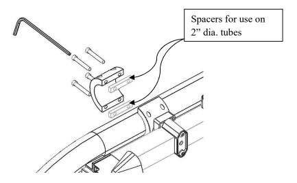
Place the LS&B with partial clamps against the tube and loosely install clamp back and spacers, if required for your tube diameter.
