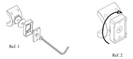
As shownt in Ref. 1 above, loosely assemble the components shown for both clamps. When assembled, the lower clamp body should be able to rotate lightly (Ref. 2). <u>DO NOT</u> tighten firmly.
