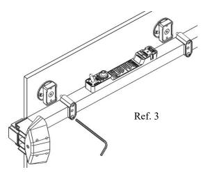
Place the U shaped upper clamps over the LS&B and firmly install the four mounting screws (Ref. 3)
