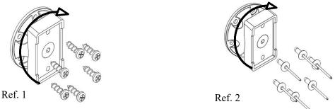
Install the fasteners by rotating the clamp base to expose the holes referenced in 1 and 2 above.
